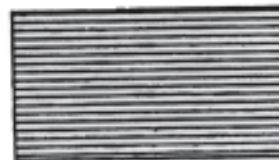
Fig 5 : Closed Picked Stone Surface
